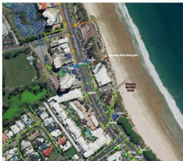
Figure 8. Synoptic Scale View of Stormwater Network (green and orange lines) and Monitored Assets (blue points) around the Cigarette Butt Voting Bin (red pin)
