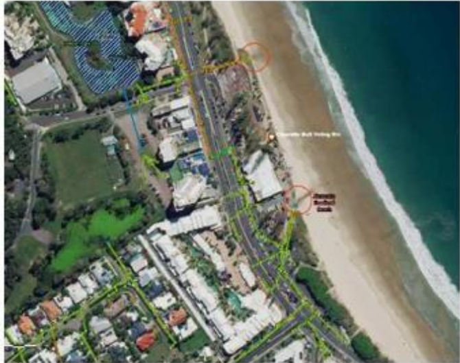
Figure 4. Map of Stormwater Pipes (green and orange lines), Drains (green and orange squares) and Outlets (circled in red on the beach) around Alex Surf Club (accessed using Sunshine Coast Council GIS Layers, 2019)
